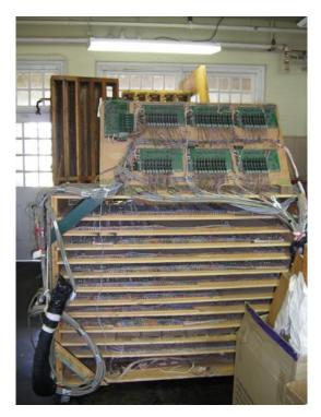
Figure 10 Devtronix Organ Relay
