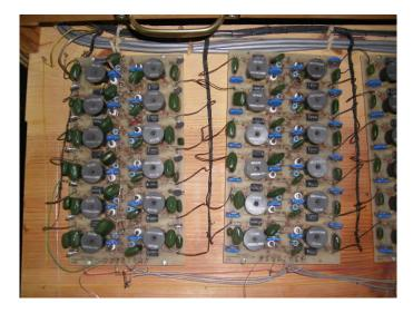
Figure 9 Oscillator Boards
