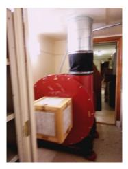
Figure 27 Air Filter on Intake
